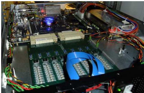
Fig. 4. The ROACH1 board, a XILINX Virtex-5 SX95T FPGA board, with the 64 input ADC connected via two Z-DOK connectors.
